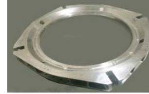
Rotor Mast Bearing Housing - Titanium
