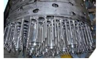
Control Plug for Reactor
