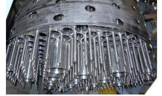
Control Plug for Reactor
