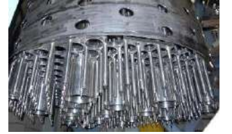
Control Plug for Reactor
